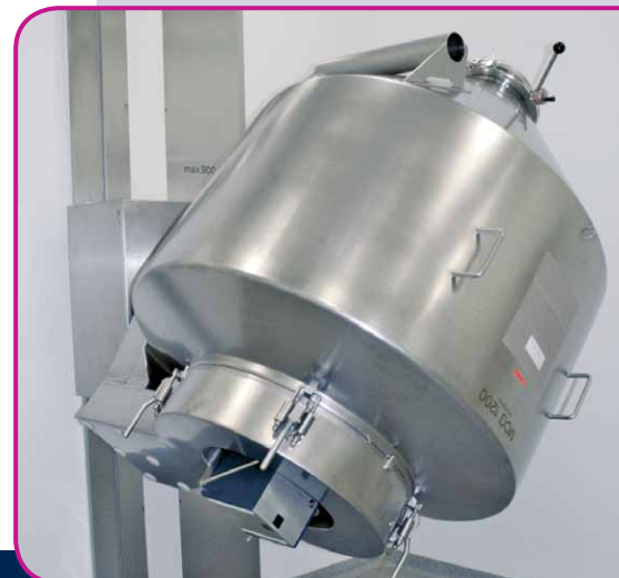
IBC equipped with SentroPAT BU II
